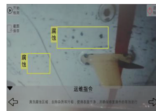
(e) 腐蚀检测
